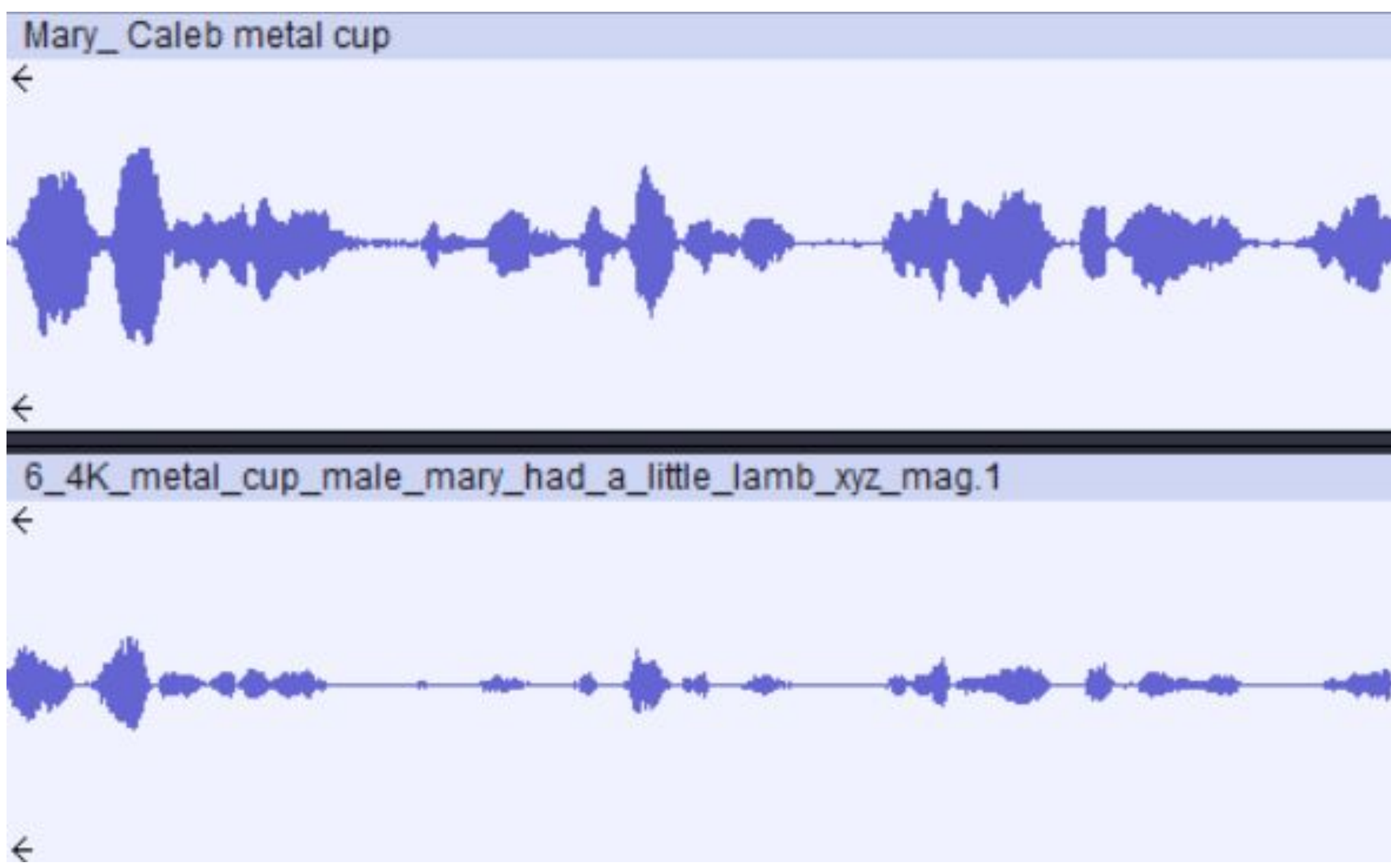
Figure 7: Displays how the accelerometer data is processed. Upper line is the audio recorded by a microphone and the lower line is the accelerometer recorded audio.
